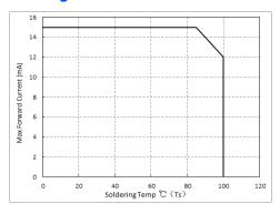
Max Driving Forward Current vs. Soldering Temp
